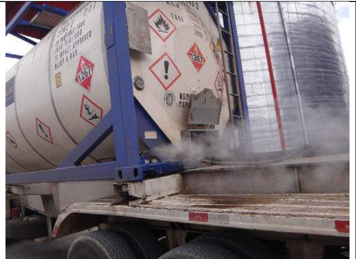
16. Steam to isotainer at Tank 117 during offloading
