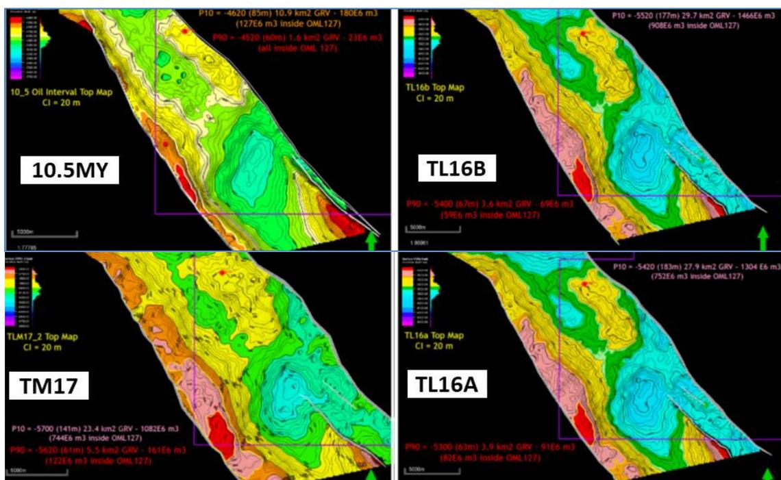
Figure 3-8: Top reservoir depth structure maps (2016/2017)
