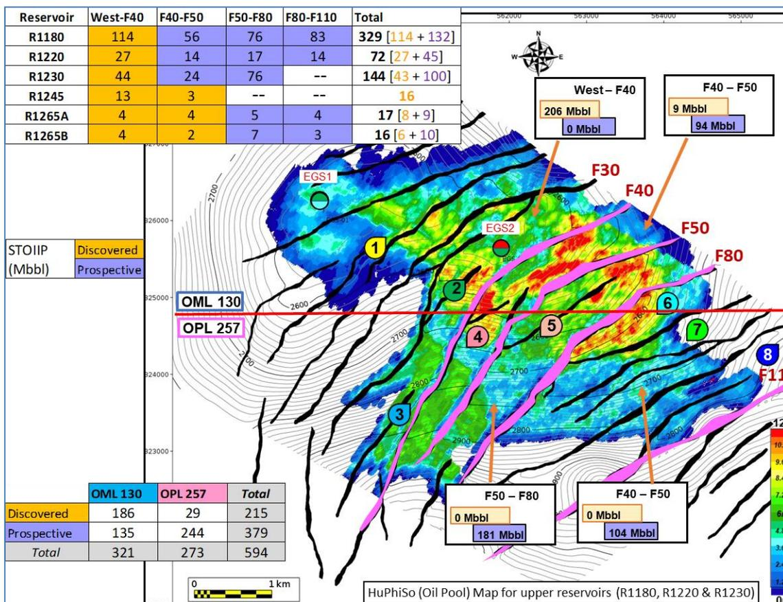
Figure 5-3: Egina South A Top Reservoir Depth Map, discovered and undiscovered STOIIP.
